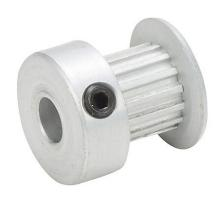
SureMotion timing pulley, aluminum, 0.08in MXL pitch, 15 tooth, 0.382in pitch diameter, 3/16in bore, oversize hub with flange. For use with 1/4in wide belt.
