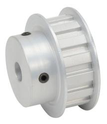
SureMotion timing pulley, aluminum, 3/8in L pitch, 15 tooth, 1.79in pitch diameter, 3/8in bore, hub with flanges. For use with 1/2in wide belt.
