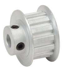
SureMotion timing pulley, aluminum, 1/5in XL pitch, 14 tooth, 0.891in pitch diameter, 1/4in bore, hub with flanges. For use with 3/8in wide belt.
