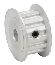
SureMotion timing pulley, aluminum, 1/5in XL pitch, 14 tooth, 0.891in pitch diameter, 1/4in bore, no hub with flanges. For use with 3/8in wide belt.
