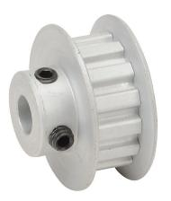
SureMotion timing pulley, aluminum, 1/5in XL pitch, 14 tooth, 0.891in pitch diameter, 1/4in bore, hub with flanges. For use with 1/4in wide belt.
