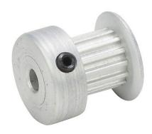
SureMotion timing pulley, aluminum, 0.08in MXL pitch, 14 tooth, 0.357in pitch diameter, 1/8in bore, oversize hub with flange. For use with 1/4in wide belt.
