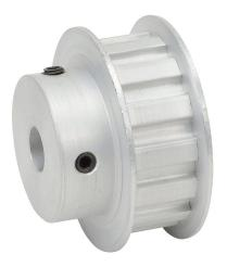
SureMotion timing pulley, aluminum, 3/8in L pitch, 14 tooth, 1.671in pitch diameter, 3/8in bore, hub with flanges. For use with 1/2in wide belt.
