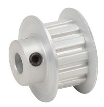
SureMotion timing pulley, aluminum, 1/5in XL pitch, 13 tooth, 0.828in pitch diameter, 1/4in bore, hub with flanges. For use with 3/8in wide belt.
