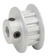
SureMotion timing pulley, aluminum, 1/5in XL pitch, 13 tooth, 0.828in pitch diameter, 1/4in bore, hub with flanges. For use with 1/4in wide belt.
