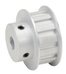
SureMotion timing pulley, aluminum, 3/8in L pitch, 13 tooth, 1.552in pitch diameter, 3/8in bore, hub with flanges. For use with 1/2in wide belt.
