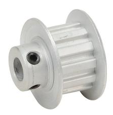
SureMotion timing pulley, aluminum, 1/5in XL pitch, 12 tooth, 0.764in pitch diameter, 1/4in bore, hub with flanges. For use with 3/8in wide belt.
