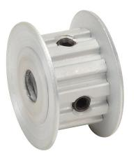
SureMotion timing pulley, aluminum, 1/5in XL pitch, 12 tooth, 0.764in pitch diameter, 1/4in bore, no hub with flanges. For use with 3/8in wide belt.
