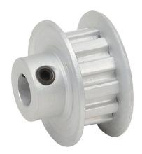
SureMotion timing pulley, aluminum, 1/5in XL pitch, 12 tooth, 0.764in pitch diameter, 1/4in bore, hub with flanges. For use with 1/4in wide belt.
