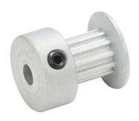
SureMotion timing pulley, aluminum, 0.08in MXL pitch, 12 tooth, 0.306in pitch diameter, 1/8in bore, oversize hub with flange. For use with 1/4in wide belt.
