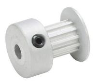
SureMotion timing pulley, aluminum, 0.08in MXL pitch, 12 tooth, 0.306in pitch diameter, 1/8in bore, oversize hub with flange. For use with 1/4in wide belt.
