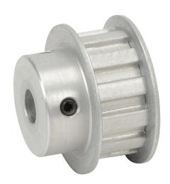
SureMotion timing pulley, aluminum, 3/8in L pitch, 12 tooth, 1.432in pitch diameter, 3/8in bore, hub with flanges. For use with 1/2in wide belt.
