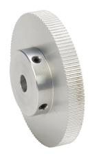
SureMotion timing pulley, aluminum, 0.08in MXL pitch, 120 tooth, 3.056in pitch diameter, 3/8in bore, hub without flanges. For use with 1/4in wide belt.
