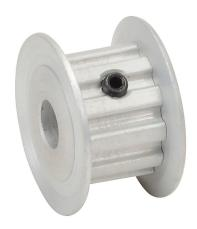
SureMotion timing pulley, aluminum, 1/5in XL pitch, 11 tooth, 0.7in pitch diameter, 1/4in bore, no hub with flanges. For use with 3/8in wide belt.
