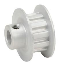
SureMotion timing pulley, aluminum, 1/5in XL pitch, 11 tooth, 0.7in pitch diameter, 1/4in bore, hub with flanges. For use with 1/4in wide belt.
