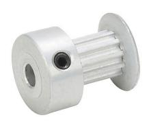
SureMotion timing pulley, aluminum, 0.08in MXL pitch, 11 tooth, 0.28in pitch diameter, 1/8in bore, oversize hub with flange. For use with 1/4in wide belt.
