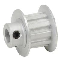
SureMotion timing pulley, aluminum, 1/5in XL pitch, 10 tooth, 0.637in pitch diameter, 1/4in bore, hub with flanges. For use with 3/8in wide belt.
