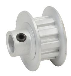
SureMotion timing pulley, aluminum, 1/5in XL pitch, 10 tooth, 0.637in pitch diameter, 1/4in bore, hub with flanges. For use with 1/4in wide belt.
