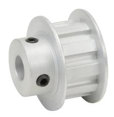
SureMotion timing pulley, aluminum, 3/8in L pitch, 10 tooth, 1.194in pitch diameter, 3/8in bore, hub with flanges. For use with 1/2in wide belt.
