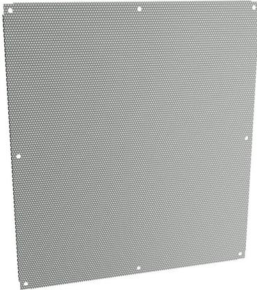
Hammond subpanel, perforated, carbon steel, ANSI 61 gray, powder coat finish. For use with 36x30 (HxW) N1A3630xx enclosures.
