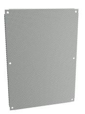
Hammond subpanel, perforated, carbon steel, ANSI 61 gray, powder coat finish. For use with 30x20 (HxW) N1A3020x enclosures.
