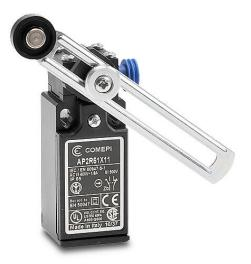
Comepi safety limit switch, side rotary adjustable lever with nylon roller, (1) N.C. safety output(s), (1) N.O. monitoring output(s), slow action break before make, plastic, (1) PG11 cable entry with 1/2in NPT adapter.
