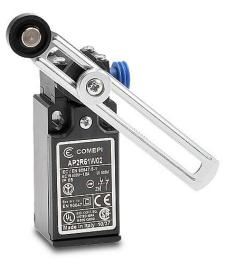
Comepi safety limit switch, side rotary adjustable lever with nylon roller, (2) N.C. safety output(s), slow action, plastic, (1) PG11 cable entry with 1/2in NPT adapter.
