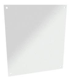
Hammond subpanel, carbon steel, RAL 9003 white, powder coat finish. For use with 24x20 (HxW) N1A2420xx enclosures.
