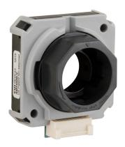
Same Sky AMT33 series incremental (quadrature)/commutation rotary modular kit encoder, 5 VDC, radial exit, line driver (differential) encoder output, up to 4096 ppr, software configurable, line driver (differential) commutation output.
