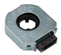
Same Sky AMT31 series incremental (quadrature)/commutation rotary modular kit encoder, 5 VDC, radial exit, line driver (differential) encoder output, up to 4096 ppr, software configurable, line driver (differential) commutation output.
