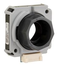
Same Sky AMT13 series incremental (quadrature) rotary modular kit encoder, 5 VDC, radial exit, push-pull (totem) output, up to 4096 ppr, software configurable. For use with NEMA 34 dual shaft motors.
