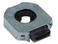
CUI Devices AMT11 series incremental (quadrature) rotary modular kit encoder, 5 VDC, radial exit, push-pull (totem) output, up to 4096 ppr, software configurable. For use with NEMA 14, 17, and 23 dual shaft motors.
