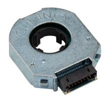
Same Sky AMT11 series incremental (quadrature) rotary modular kit encoder, 5 VDC, radial exit, line driver (differential) output, up to 4096 ppr, software configurable. For use with NEMA 14, 17, and 23 dual shaft motors.
