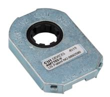
CUI Devices AMT10 series incremental (quadrature) rotary modular kit encoder, 5 VDC, radial exit, push-pull (totem) output, up to 2048 ppr, dipswitch configurable. For use with NEMA 14, 17, and 23 dual shaft motors.
