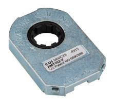
Same Sky AMT10 series incremental (quadrature) rotary modular kit encoder, 5 VDC, radial exit, push-pull (totem) output, up to 2048 ppr, dipswitch configurable. For use with NEMA 14, 17, and 23 dual shaft motors.
