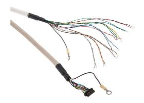
CUI Devices encoder cable, 17-pin connector to pigtail, shielded, twisted pair, 10ft cable length. For use with CUI Devices AMT112 and AMT312 encoders.
