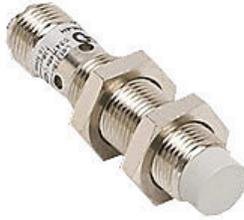
Micro Detectors inductive proximity sensor, tubular, 12mm diameter x 52.5mm body, nickel-plated brass housing, PNP, N.O. output, 8mm sensing distance, non-flush, 2 kHz switching frequency, IP67, 4-pin M12 quick-disconnect.
