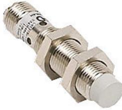
Micro Detectors inductive proximity sensor, tubular, 12mm diameter x 52.5mm body, nickel-plated brass housing, NPN, N.O. output, 8mm sensing distance, non-flush, 2 kHz switching frequency, IP67, 4-pin M12 quick-disconnect.
