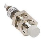
Micro Detectors inductive proximity sensor, tubular, 12mm diameter x 44mm body, nickel-plated brass housing, NPN, N.O. output, 8mm sensing distance, non-flush, 2 kHz switching frequency, IP67, pigtail.
