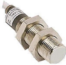
Micro Detectors inductive proximity sensor, tubular, 12mm diameter x 44mm body, nickel-plated brass housing, NPN, N.O. output, 4mm sensing distance, flush, 2 kHz switching frequency, IP67, pigtail.
