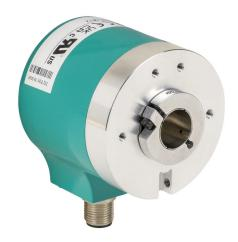
Lika Electronic AM59 series multi-turn absolute rotary encoder, 10-30 VDC, Modbus RTU output, medium duty, up to 13-bit (8192 ppr)/up to 14-bit turns, multiple hollow shafts (6mm - 15mm), 58mm diameter body, IP65, radial exit, M12 male.
