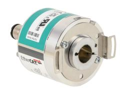
Lika Electronic AM59 series multi-turn absolute rotary encoder, 5-30 VDC, EtherCAT output, medium duty, up to 13-bit (8192 ppr)/up to 14-bit turns, multiple hollow shafts (6mm - 15mm), 58mm diameter body, IP65, axial exit, M12 male.
