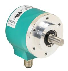
Lika Electronic AM58 series multi-turn absolute rotary encoder, 10-30 VDC, Modbus RTU output, medium duty, up to 13-bit (8192 ppr)/up to 14-bit turns, 3/8in solid shaft, 58mm diameter body, IP65, radial exit, M12 male.
