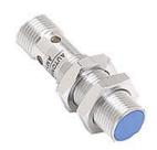
AutomationDirect inductive proximity sensor, tubular, 12mm diameter x 45mm body, chrome-plated brass housing, PNP, N.O. output, 6mm sensing distance, semi-flush, 800 Hz switching frequency, IP67, 4-pin M12 quick-disconnect.
