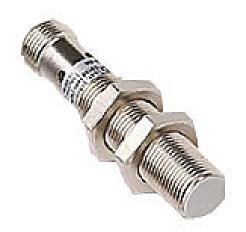
Micro Detectors inductive proximity sensor, tubular, 12mm diameter x 65mm body, nickel-plated brass housing, PNP, N.O. output, 2mm sensing distance, flush, 2 kHz switching frequency, IP67, 4-pin M12 quick-disconnect.
