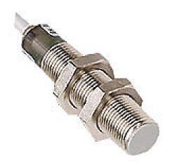
Micro Detectors inductive proximity sensor, tubular, 12mm diameter x 50mm body, nickel-plated brass housing, PNP, N.O. output, 2mm sensing distance, flush, 2 kHz switching frequency, IP67, pigtail.
