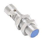
AutomationDirect inductive proximity sensor, tubular, 12mm diameter x 45mm body, chrome-plated brass housing, NPN, N.O. output, 6mm sensing distance, semi-flush, 800 Hz switching frequency, IP67, 4-pin M12 quick-disconnect.
