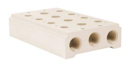
NITRA pneumatic valve manifold, aluminum, off-white, (4) stations, (2) 1/2in female NPT inlet(s), (4) 1/2in female NPT exhaust(s). For use with AVS-54 series directional control valves.
