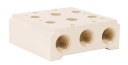
NITRA pneumatic valve manifold, aluminum, (2) stations, (2) 1/2in female NPT inlet(s), (4) 1/2in female NPT exhaust(s). For use with AVS-54 series directional control valves.
