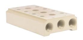
NITRA pneumatic valve manifold, aluminum, off-white, (4) stations, (2) 3/8in female NPT inlet(s), (4) 3/8in female NPT exhaust(s). For use with AVS-53 series directional control valves.
