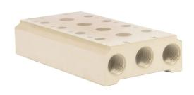
NITRA pneumatic valve manifold, aluminum, (4) stations, (2) 3/8in female NPT inlet(s), (4) 3/8in female NPT exhaust(s). For use with AVS-53 series directional control valves.
