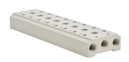
NITRA pneumatic valve manifold, aluminum, off-white, (8) stations, (2) 1/4in female NPT inlet(s), (4) 1/4in female NPT exhaust(s). For use with AVS-52 series directional control valves.
