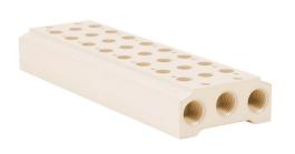
NITRA pneumatic valve manifold, aluminum, (8) stations, (2) 1/4in female NPT inlet(s), (4) 1/4in female NPT exhaust(s). For use with AVS-51 series directional control valves.
